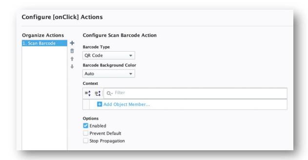
6. After clicking on OK, this will physically launch the scanning feature on the device when the component is clicked on. Next, we need to tell the session what to do with the barcode data once it has been scanned.
