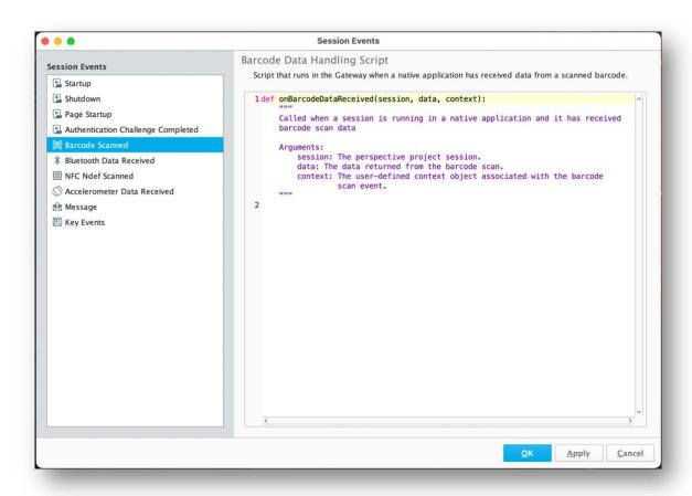
9. Firstly, we want to log the data so that we can see what it looks like. This will help to understand how the data is received and find the best way to store, manipulate and display the data afterwards. For that, we want to create a logger and log the data and context parameters:
