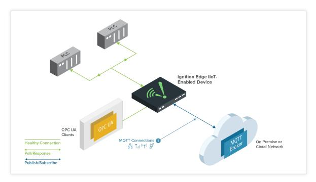
**Ignition Edge IIoT Standalone:** Use Edge IIoT as a standalone edge gateway to publish device data from the edge of the network to an MOTT broker.
