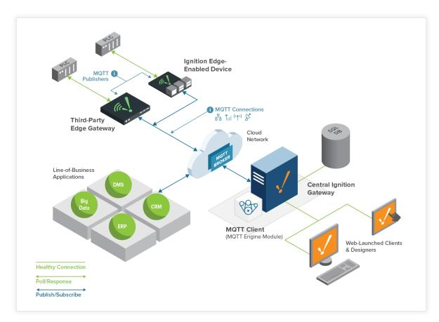
Ignition Edge Remote IIoT: Use Edge IIoT as an edge gateway to publish device data from the edge of the network to an MQTT broker.
