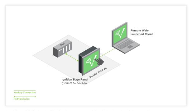
Standalone HMI: Use Ignition Edge Panel to create a standalone HMI at the edge of the network.
